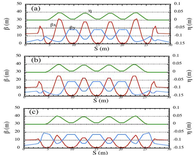
Figure 5: Optics functions in a 5-bend achromat cell for the original lattice (a), and the detuned lattices (b) (c).
