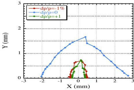
Figure 2: Dynamic aperture at the centre of a straight section.
