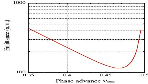
Figure 4: Relation between the phase advance and the emittance for a TME lattice.
