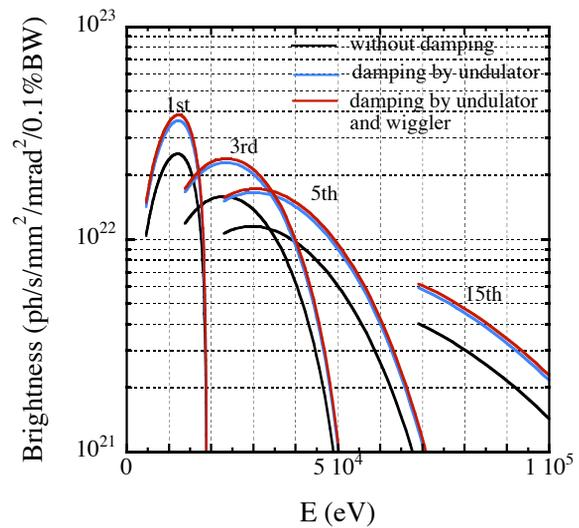
Figure 7: Brightness for a 4.5-m undulator without damping (black), damping by undulators (blue), and damping by wigglers and undulators (red).
