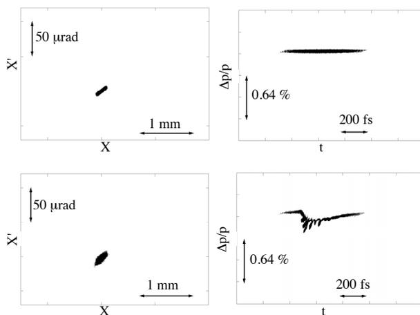
Figure 10: Transverse and longitudinal phase space distribution for CSR suppression DBA lattice without CSR (upper) and with CSR (lower).
