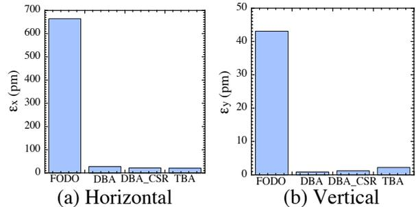
Figure 7: Emittance growth by synchrotron radiation.
