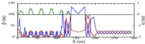
Figure 5: Optics functions of DBA based beam transport line. Phase advance is chosen to suppress the CSR effects.
