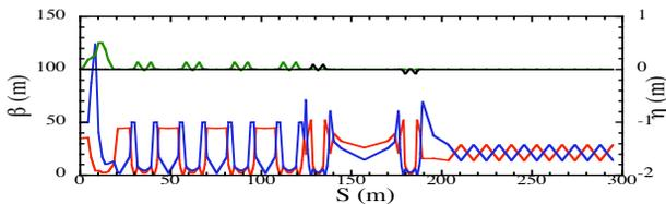
Figure 6: Optics functions of TBA based transport line.
