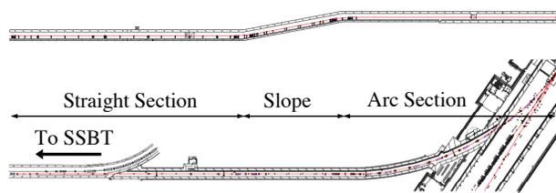
Figure 2: Beam transport line from the SACLA linac to the SSBT (XSBT).
