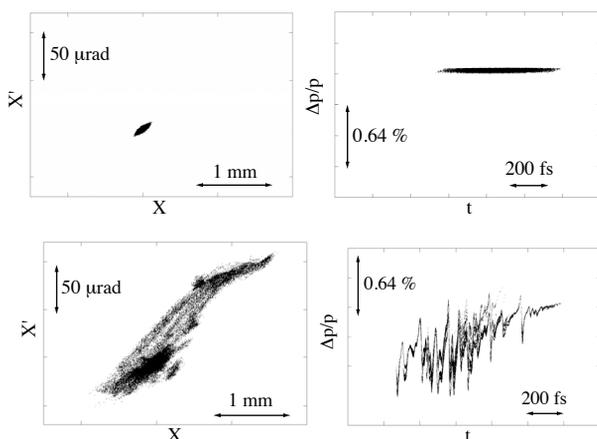
Figure 9: Transverse and longitudinal phase space distribution for simple DBA based beam transport line without CSR (upper) and with CSR (lower).
