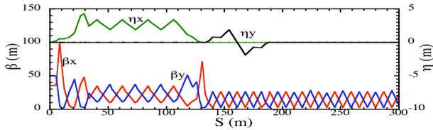
Figure 3: Optics functions of FODO based beam transport line.
