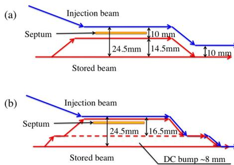
Figure 2: (a) Off- and (b) on-axis injection setups.
