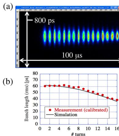
Figure 3: (a) Streak image and (b) bunch distributions turn by turn.
