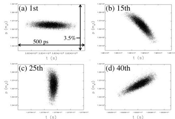
Figure 1: Longitudinal beam distributions at (a) 1st, (b) 15th, (c) 25th, and (d) 40th turns. Horizontal axis is time and vertical axis is momentum deviations. Full scales of each axis correspond to  $\Delta t = 500$  ps horizontally and  $\Delta E/E = 3.5\%$  vertically.
