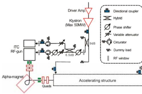
Figure 2: High power waveguide circuit for the t-ACTS injector.
