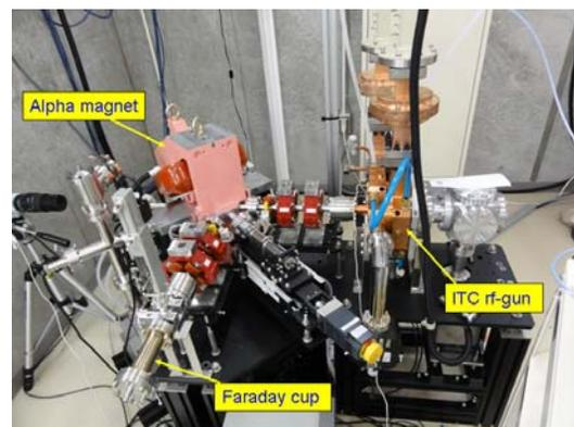
Figure 1: Present t-ACTS injector beam line.
