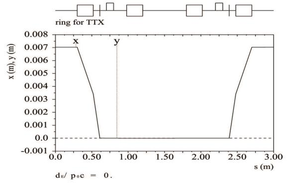
Figure 3: The closed orbit at the beam injection.
