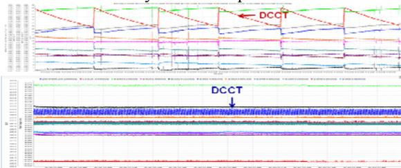
Figure 8: BPM records horizontal orbit drift for decay (up) and top-up (below) operation.
