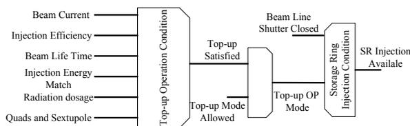
Figure 3: Top-up operation interlock logic diagram.
