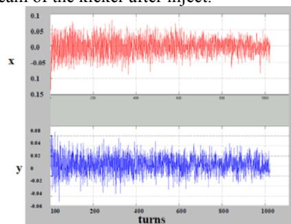
Figure 5: BPM turn-by-turn data after injection.
