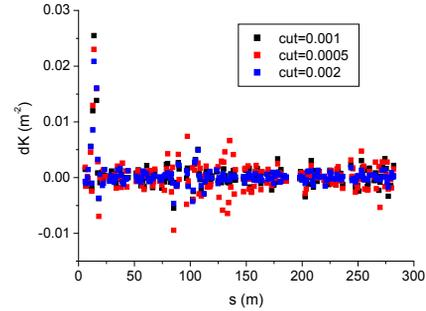
Figure 3: Quadrupole correction strengths corresponding to the single known error for various SVD cut.
