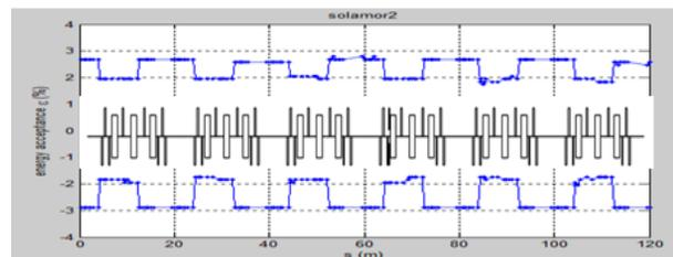
Figure 5: Energy acceptance along the ring with 1% coupling and multipole error.
