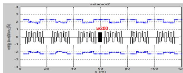
Figure 7: Top: dynamic aperture, bottom: momentum acceptance along the ring with 1% coupling. Wiggler W200 was included.
