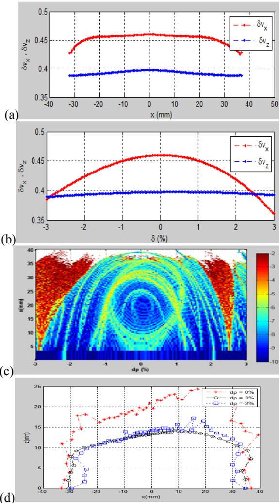
Figure 3: (a) tune shift vs. amplitude (b) tune shift vs. momentum (c) frequency map analysis (x v.s. dp/p) (d) dynamic aperture. The tracking simulations were done with chromaticity  $\xi_x/\xi_y = 0.095/0.065$
