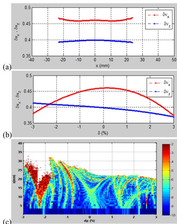
Figure 6: (a) tune shift vs. amplitude (b) tune shift vs. momentum (c) frequency map analysis (x v.s. dp/p), wiggler W200 was included.
