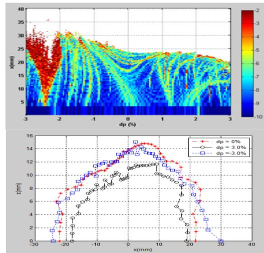
Figure 4: Top: frequency map analysis (x v.s. dp/p), bottom: dynamic aperture  $\xi_x/\xi_y = 0.095/0.065$ . Multipole errors were included in the tracking simulations
