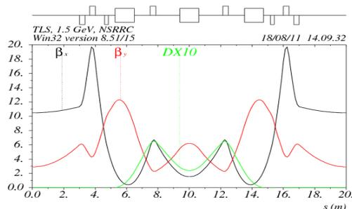
Figure 1: Lattice function of TLS storage ring for one period (TBA lattice).
