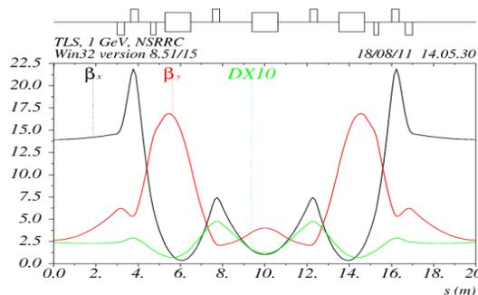
Figure 2: Lattice function of TLS storage ring for one period (non-achromatic low-emittance mode).
