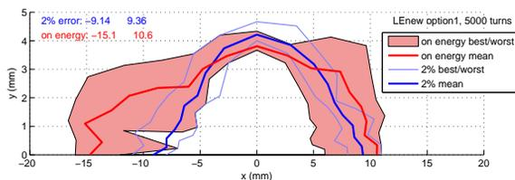
Figure 2: Dynamic aperture of the optimized lattice with working point [15.127, 6.224]. Systematic and random field errors and insertion device non-linearity are included. Beta beating of 1% rms and  $x/y$  coupling of 1% are created in all 15 random seeds.
