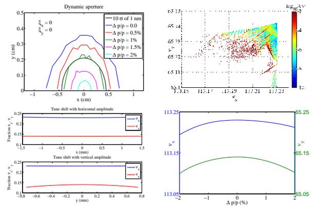
Figure 5: Dynamic aperture (upper left), tune footprint (upper right), amplitude-dependent tune (lower left) and chromatic tune (lower right) with geometric sextupoles.
