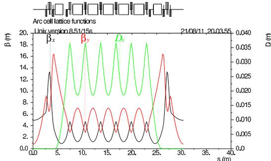
Figure 2: Lattice functions in PEP-X 7-bend achromat cell.
