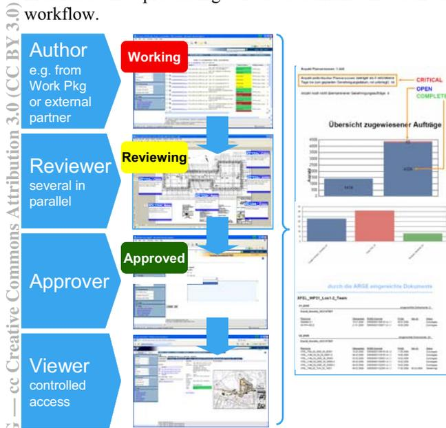
Figure 2: EDMS-based document review & approval workflow, and coordinator’s report about pending and completed processes.
