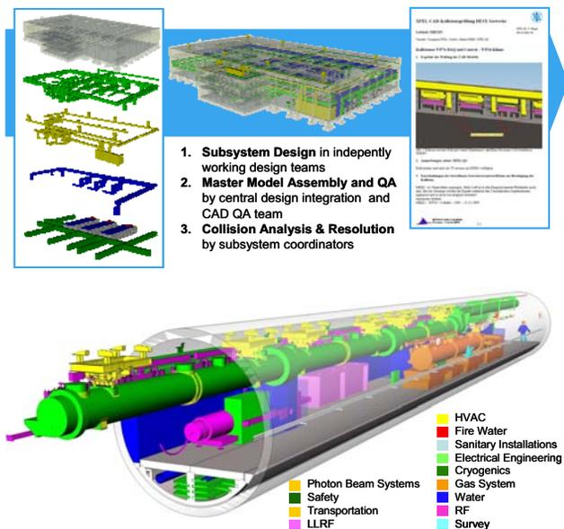
Figure 1: Master model with contributions from various disciplines (top) and collaborative design process at European XFEL
