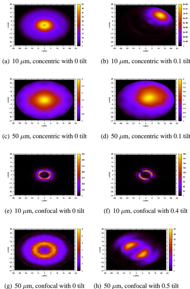
Figure 2: Contour plot of mode profile on out-coupling mirror.
