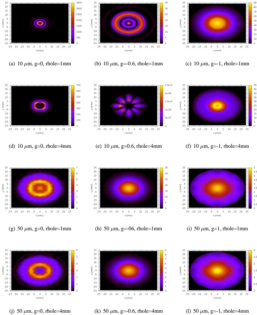
Figure 3: Contour plot of mode profile on out-coupling mirror.
