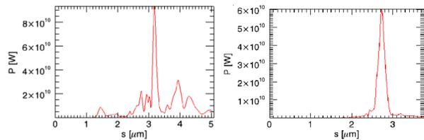
Figure 7: Simulated FEL power profile at undulator  $z=50$ m from electrons shown in Fig.6, without foil (left) and with 0.8mm width slotted foil (right).
