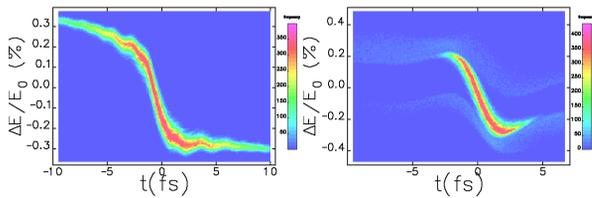
Figure 6: Longitudinal phase at the beginning of the undulator with L2 RF phase  $-33.5^\circ$ , Laser heater 6 keV and DL2  $R_{56} = 0.133$  mm. (left) without slotted foil; (right) with 0.8mm width foil.
