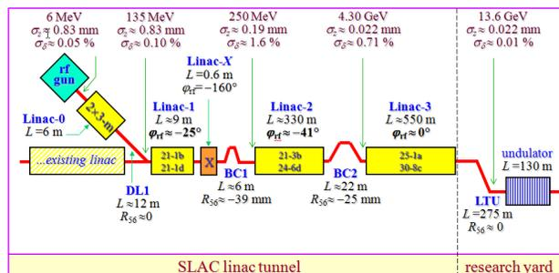
Figure 1: Layout of the LCLS machine.
