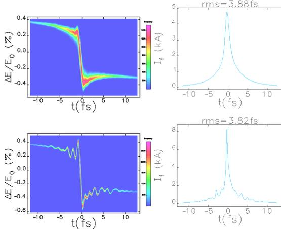
Figure 2: Laser heater effect on longitudinal phase space at undulator entrance with L2 RF phase  $-33.3^\circ$ : with laser heater 6keV (top) and without laser heater (bottom). The computation uses 12M particles and 500 bins for longitudinal space charge calculation. DL2  $R_{56} = 0.133$  mm.
