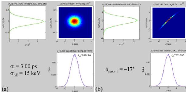
Figure 4: (a) Injected bunch at 10 MeV (b) Exit of the first pass through the linac.
