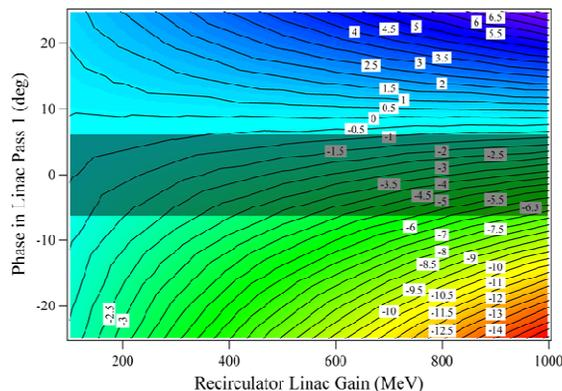
Figure 3: Contour plot showing the absolute energy spread at the photon generator (in MeV) as a function of acceleration phase in the first pass through the linac and of the energy gain in the recirculator linac.
