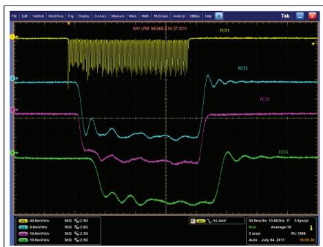
Figure 2: FCT measurements along the linac.
