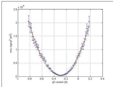
Figure 4: Typical LPM horizontal emittance measurement.
