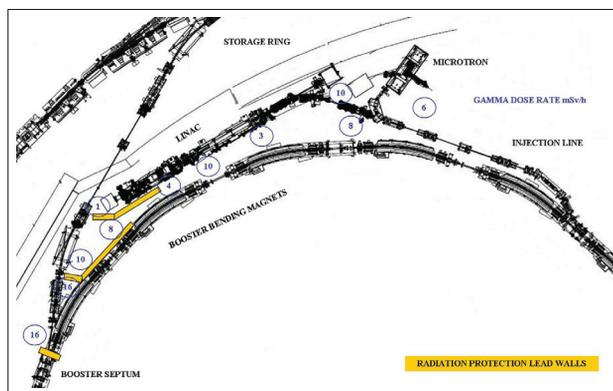
Figure 3: Radiation survey of bunker.
