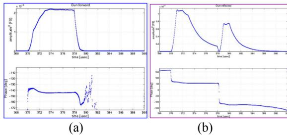
Figure 5: (a) Wave shapes of input power and input phase of RF gun and (b) wave shapes of reflected power and phase of reflected power, after optimization of reducing a level of reflected power.
