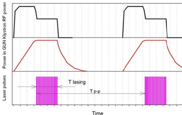
Figure 1: Shapes of first two pulses, above: output power from the klystron, high amplitude during filling time, low amplitude during flat top, middle: an electric field in the gun, bottom: a laser pulses.
