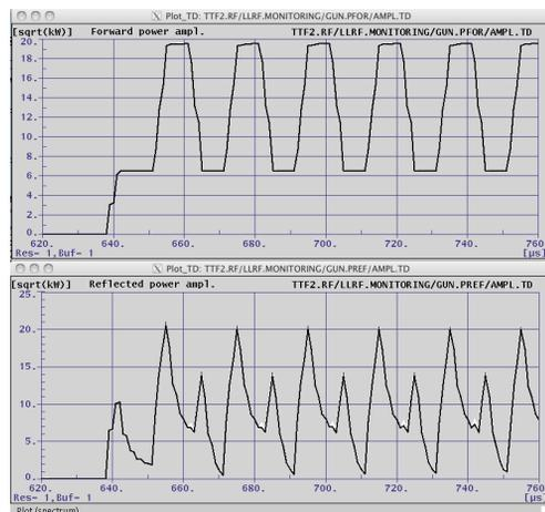
Figure 6: Wave shapes of first six from 46 pulses. Forward power (above) and reflected power (below). Data was taken with 1 MHz ADC.
