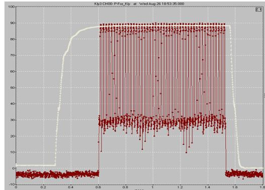
Figure 4: Example of wave shapes of klystron current (white) and output power (brown). Vertical scale is in (A) for the current and in (dBm) for klystron output power.
