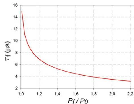
Figure 2: Total time to fill the gun cavity to the design gradient versus power ratios.
