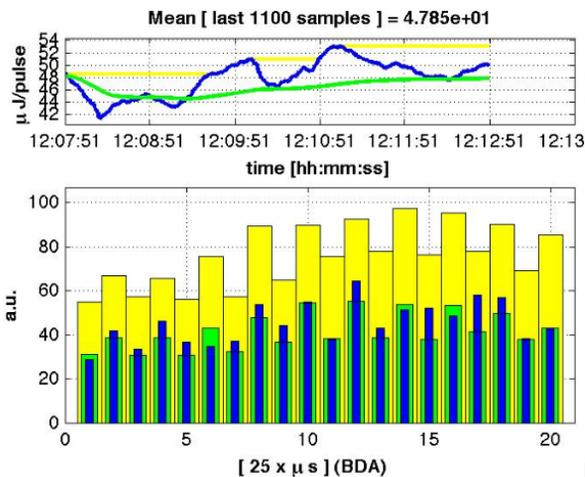
Figure 7: Photon bunch energy for 20 bunches in PIP mode of FLASH operation. Recorded with GMD detector; blue - actual pulse, green - running average, yellow - peak readings.
