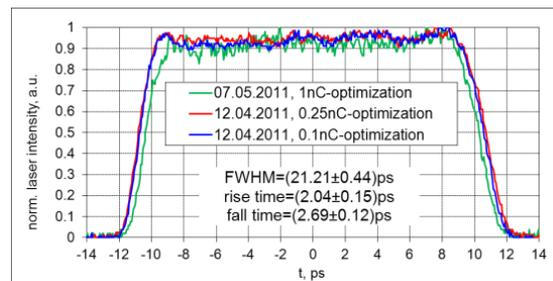
Figure 1: Temporal profiles of a photo cathode laser pulse. Each profile corresponds to the measured emittance optimum for a given bunch charge.
