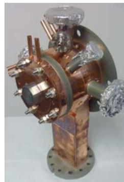
Figure 7: New photocathode RF gun after completing cold testing.
