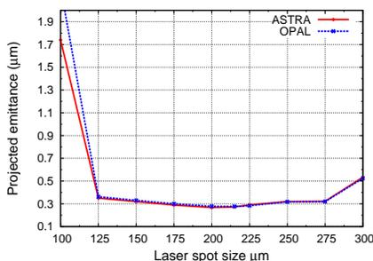
Figure 7: Projected emittance at the injector output as function of the laser spot size
