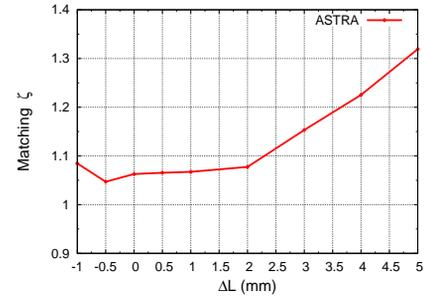
Figure 5: Matching vs half cell length variation
