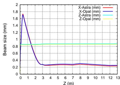
Figure 9: Longitudinal and transverse beam size along the injector
