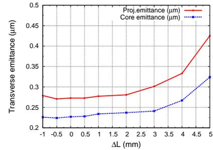
Figure 4: Emittance vs half cell length variation
