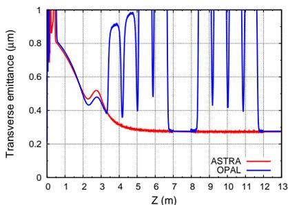
Figure 8: Projected emittance along the injector
