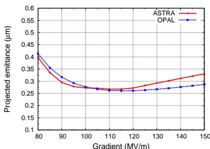
Figure 6: Projected emittance at the injector output as function of the gun gradient
