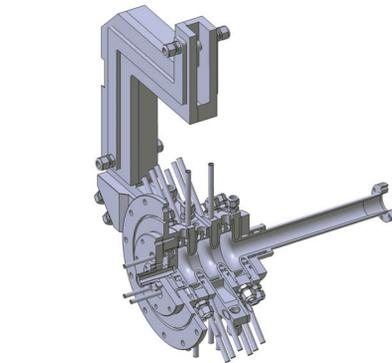
Figure 2: A 3D view of the SwissFEL RF gun
