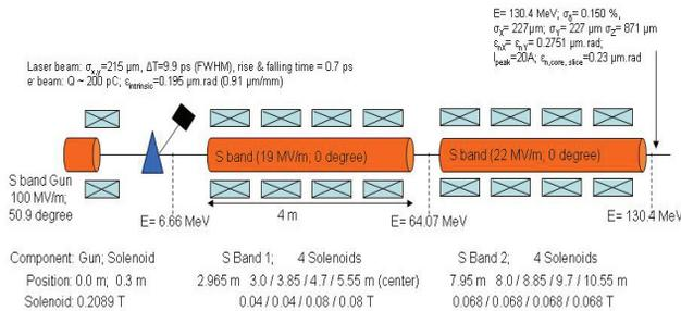
Figure 1: The low energy section of the SwissFEL
