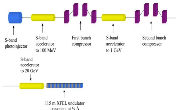
Figure 2: Preliminary layout of 50-keV XFEL 20-GeV electron linac.
