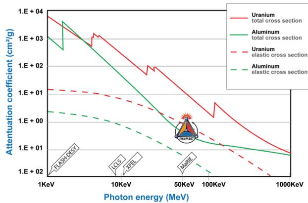
Figure 1: Photon absorption and coherent scattering coefficients for uranium and aluminium. Photon adsorption leads to sample heating, and the elastically scattered fraction gives scattering information.
