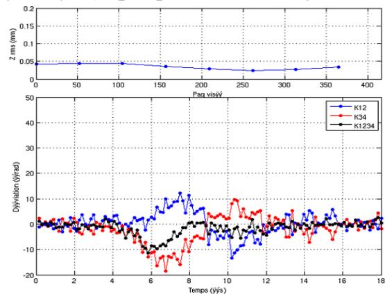
Figure 2: In Vertical plane, RMS residual oscillation (up) and kickers deviations (down).
