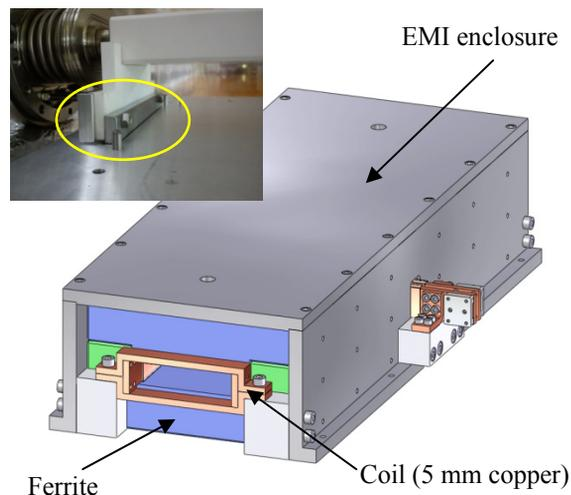
Figure 4: Kicker prototype engineering drawing and gap between kicker magnet and ceramic chamber.
