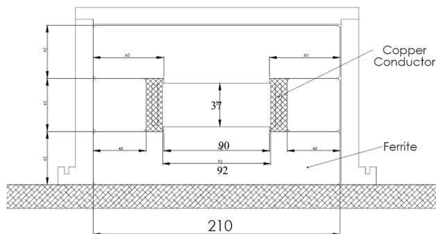
Figure 2: TPS SR kicker coil and ferrite.
