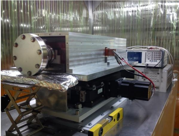
Figure 5: Kicker prototype completion and inductance measurement.
