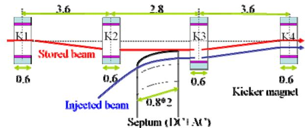
Figure 1: TPS SR Injection scheme.
