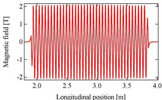
Figure 6: Measured field at minimum gap of 5.5 mm.
