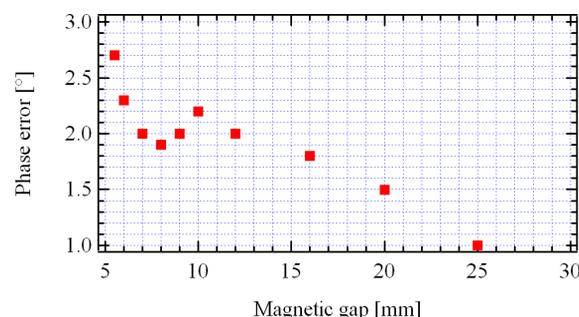
Figure 4: Phase error versus the magnetic gap.
