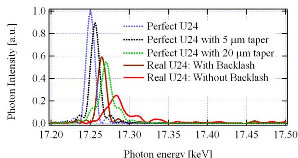
Figure 5: Effect of the backlash at 8 mm gap on the spectrum (17<sup>th</sup> harmonic) computed from the magnetic measurements (plain lines) and the effect of a taper between girders (dashed lines).
