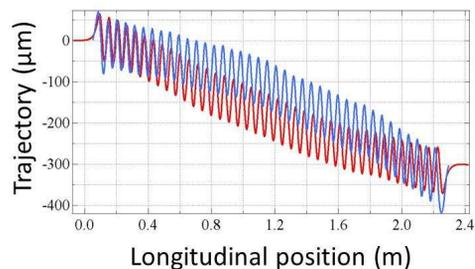
Figure 5: Measurements of the *WSV50* undulator. Hall probe measurements in red line, pulsed wire in blue. Pulse time duration fixed at  $10\text{ ms}$  with an amplitude of  $0.2\text{ A}$ .
