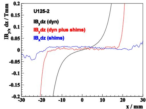
Figure 3: Dynamic vertical field integrals (dyn) before shimming (black) and with shims (red). The horizontal field integrals due to the shims are indicated in blue.
