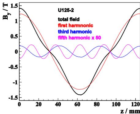
Figure 1: Total  $B_y$  and individual field harmonics of the BESSY II U125-2 plotted versus the  $z$ -direction.
