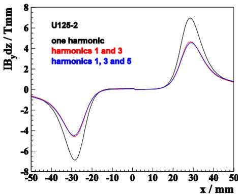
Figure 2: Dynamic field integrals of the U125-2 installed at BESSY II at smallest gap of 15.7mm. The dynamic field integrals have been determined from  $m=1, 2$  and 3 transverse profiles yielding the harmonics 1, 1 and 3 and 1, 3 and 5 (Eq. (6)). The 3<sup>rd</sup> harmonic contributes only little, however, it must be determined from Eq. (6) with  $m=2$  for a correct evaluation of the 1<sup>st</sup> harmonic.
