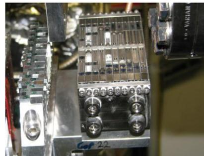
Figure 4: Permanent magnets for the compensation of dynamic field integrals at the downstream end of the BESSY II U125-2 (for details see text).
