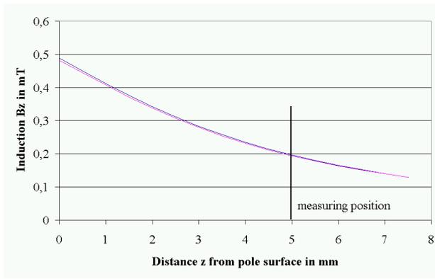
Figure 6: Induction above the pole faces of an A2-magnet.
