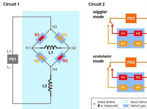
Figure 4: Measurement setup used to test the SCS built to work under conduction cooled conditions.
