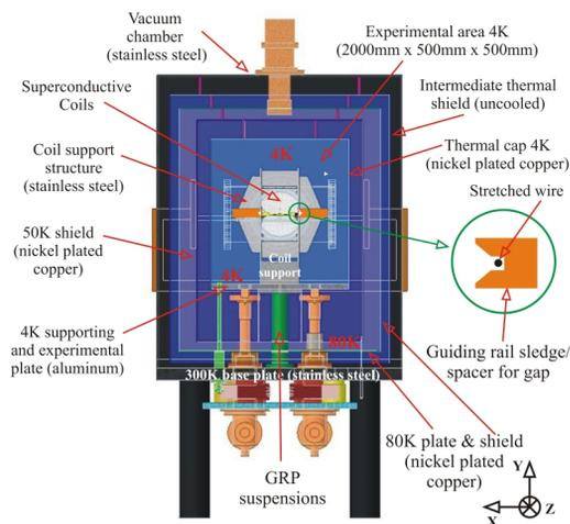
Figure 1: Sectional view from the front of the cryostat showing the different temperature regions.
