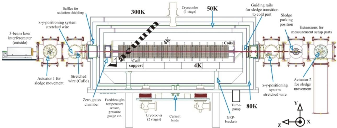
Figure 2: Drawing of the cryostat CASPER II with equipment for local and integral field measurements.
