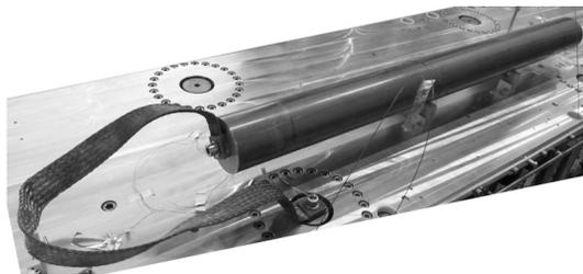
Figure 5: Picture and schematic side view of the 4K plate with FAT temperature test setup.
