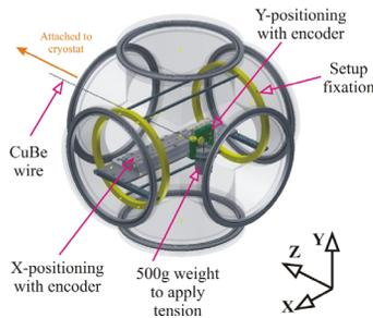
Figure 4: Measurement components for integral field measurements.
