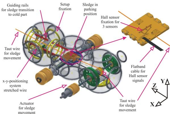
Figure 3: Drawing of the measurement parts for local field measurements.
