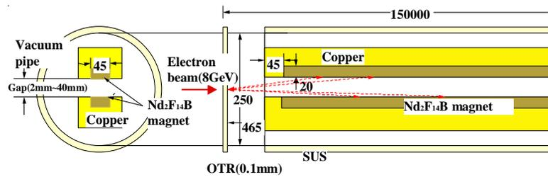
Figure 1: Geometry of simulations. (unit: mm).
