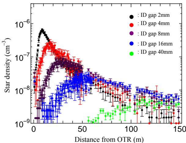
Figure 2: Star density dependence within the magnets on the gap width of ID due to 8GeV electrons injected into OTR. (Black: gap width 2mm, Red;4mm, Purple; 8mm, Blue; 16mm, Green; 40mm).
