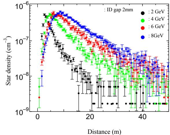
Figure 3: Star density distributions depending on electron energy within the magnet of ID. (Black; electron energy 2GeV, Green; 4GeV, Red; 6GeV, Blue; 8GeV).
