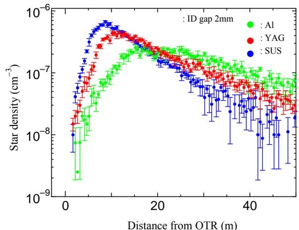
Figure 4: Star density distribution for the dependence on the material of OTR with 0.1mm thick.
