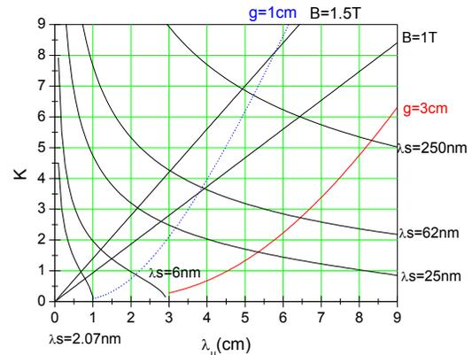
Figure 1: The relation of undulator period and deflection parameter K.
