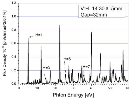
Figure 5: Flux of modified QPU88.
