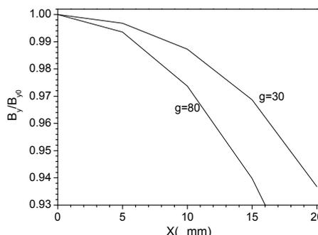
Figure 4: The transverse distribution of horizontal and vertical magnetic field for circular polarization mode.
