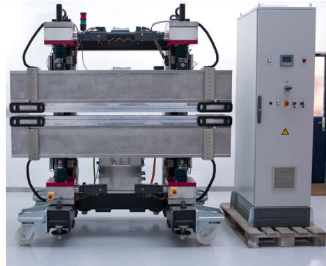
Figure 1: Finished modulator for the FEL-2 beam line, just before shipment to the FERMI@Elettra site.
