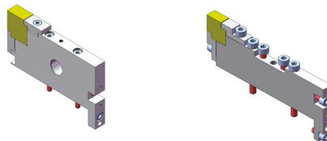
Figure 5: Old (left) and new (right) holder design. New holder ensures better stiffness to reduce the movements of the magnet blocks due to the changing magnetic forces.
