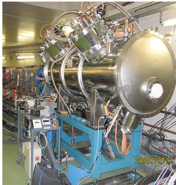
Figure 1: Superconducting wiggler installed in final position at ALBA Storage Ring is being pumped down.
