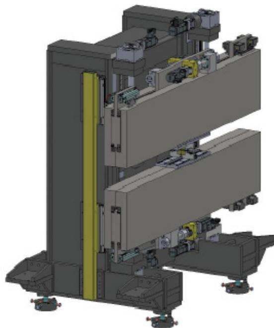
Figure 5: 3D-CAD rendering of an APPLE-II-type undulator with four moveable arrays
