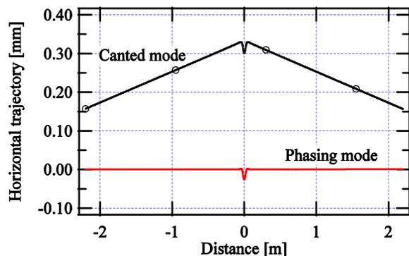
Figure 3: Electron trajectory in the straight section for the canted (line with markers) and phasing mode (line).
