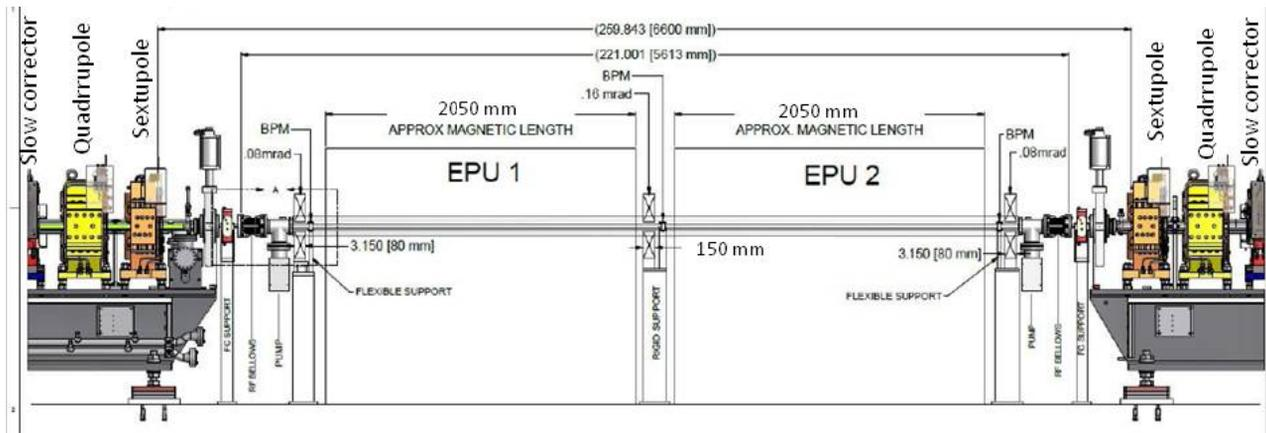
Figure 1: Layout of the CSX straight section.
