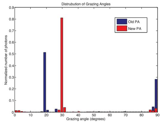
Figure 5: The grazing angle of photons incident on the PA.
