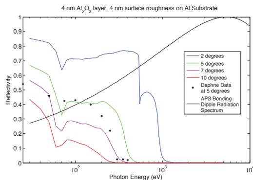
Figure 1: An example of the reflectivity of photons on a specified surface. All angles are grazing angles. Data was taken from the Berkeley Center for X-Ray Optics [3] and Daphne [4]
