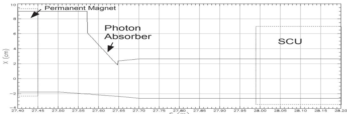
Figure 2: The design for the new PA. As shown, there is a HPM undulator before the PA and between the PA and the SCU there is room for a gate valve and a corrector magnet so that each of the undulators can be used independently.
