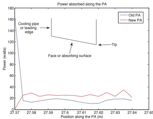
Figure 4: The power distributed along the length of the PA.
