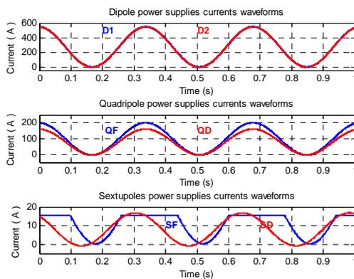
Figure 3: Waveforms of dipole (top), quadrupole (middle) and sextupole (bottom) power supplies.
