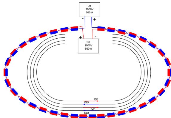
Figure 2: Power supplies connections of dipole (D1, D2), quadrupole (QF, QD), and sextupole (SF, SD) magnets.
