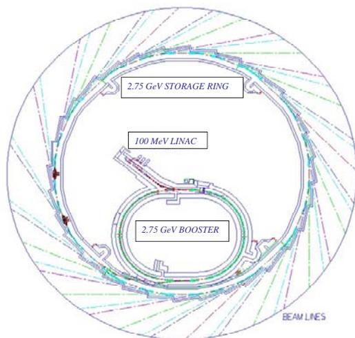
Figure 1: Layout of the SOLEIL accelerators: linac, booster, storage ring, and beam-lines.
