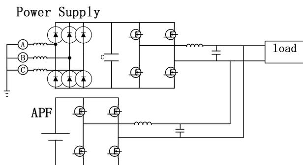
Figure 1: Single-phase APF used in AC power supply.
