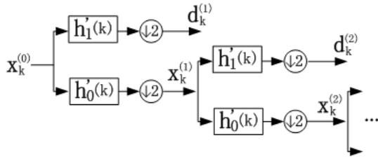
Figure 3: Process of discrete wavelet transform.
