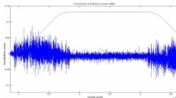
Figure 4: Reference current and tracking error.
