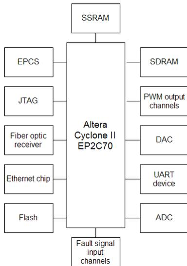
Figure 2: Hardware block diagram
