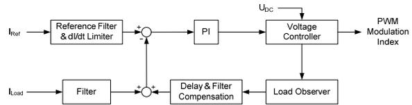
Figure 1: Simplified SS-PI controller block diagram.
