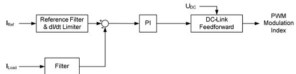
Figure 2: Simplified PI controller block diagram.
