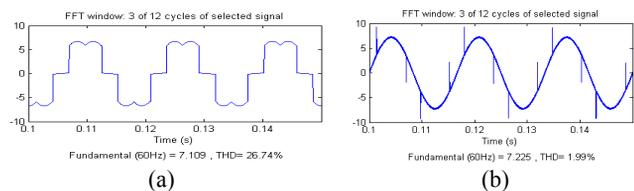
Figure 4: Simulation results (a) Normal operation (b) used the APF converter
