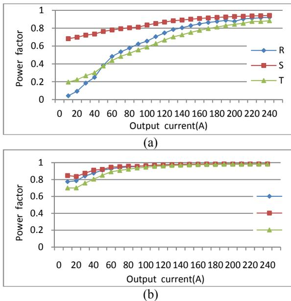
Figure 8: power factor of INVER power supply (a) Normal operation (b) used the shunt APF converter
