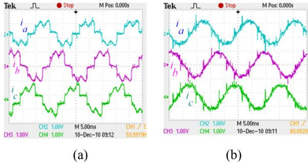
Figure 7: (a) the load current of INVER power (b) the source current of three-phase
