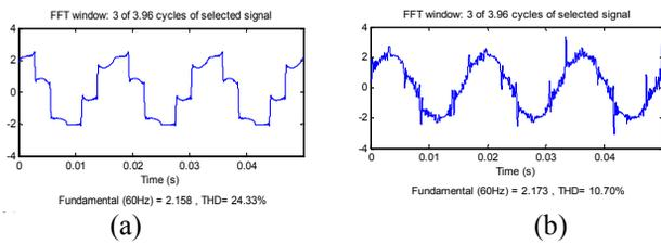
Figure 6: FFT analyze of current (a) load current; (b) source current
