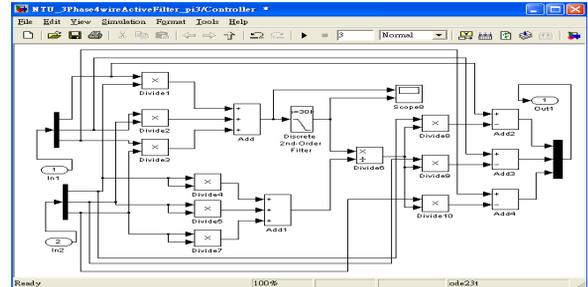
Figure 3: Current compensator internal block diagram
