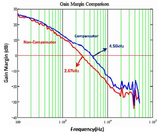
Figure 7: Open loop and close loop control to output Gain Margin bode plot.
