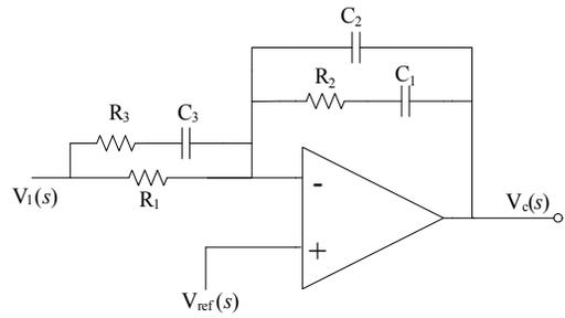
Figure 5: Compensator lead-lag equivalent circuit.
