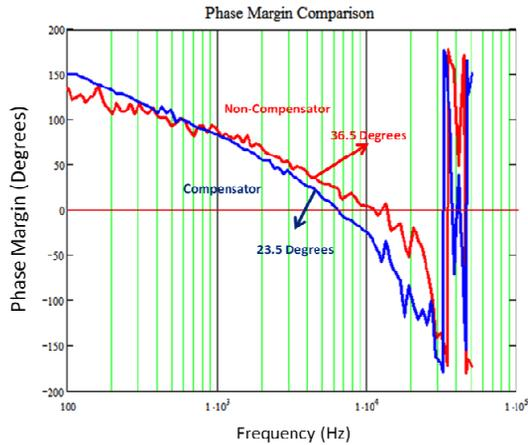
Figure 8: Open loop and close loop control to output Phase Margin bode plot.
