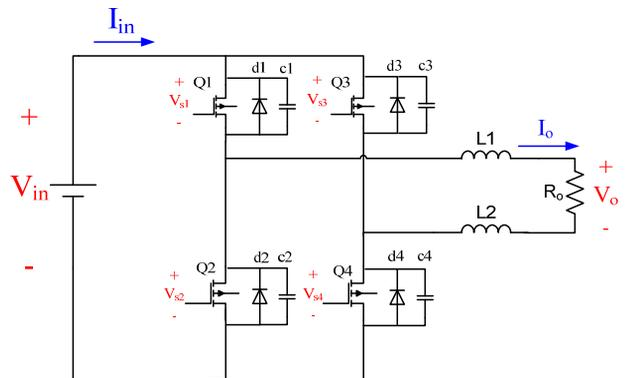
Figure 2: Correction power supply equivalent circuit.
