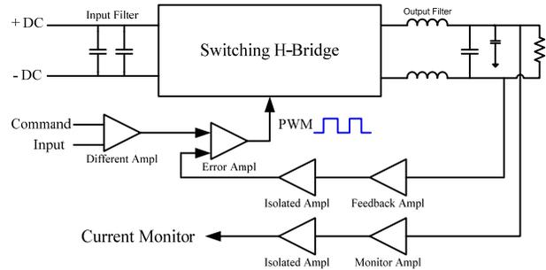
Figure 1: Correction power supply block diagram.
