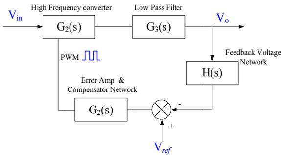
Figure 3: Correction power supply equivalent circuit.
