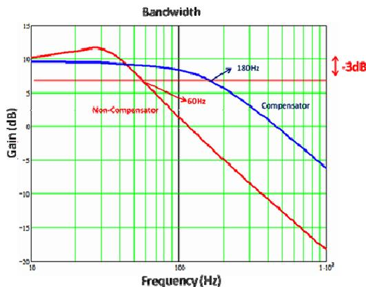
Figure 9: Compensator and non-compensator bandwidth curve.
