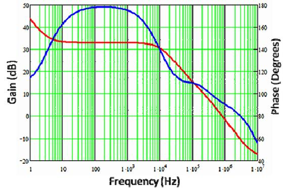
Figure 6: Simulation compensator lead-lag equivalent circuit gain margin and phase margin curve.
