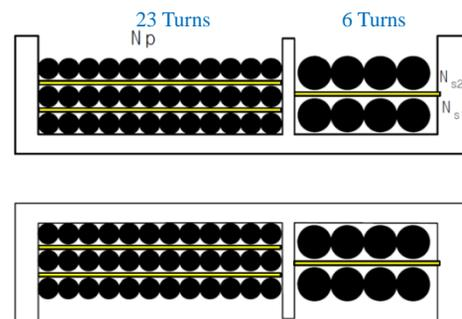
Figure 1: Fundamental structure of LLC resonant transformer.
