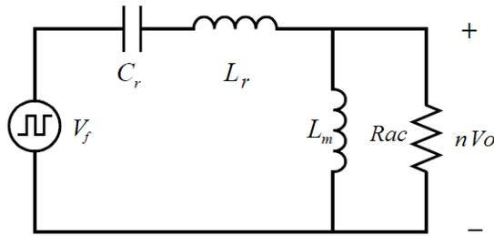
Figure 2: The structure of the LLC resonant band pass transformer.
