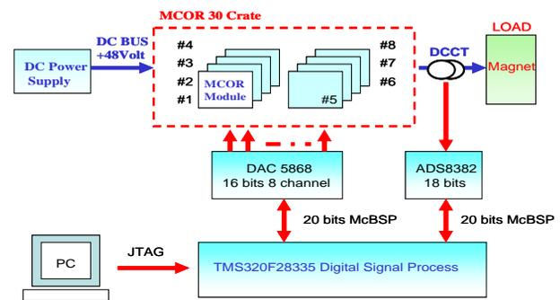
Figure 1: The structure of N+1 redundancy power converter.
