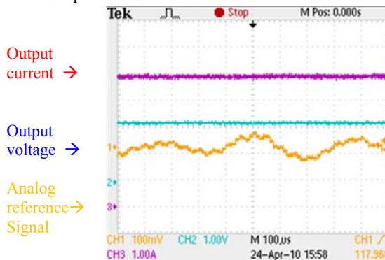
Figure 6: Reference signal and output current with voltage of close loop control.
