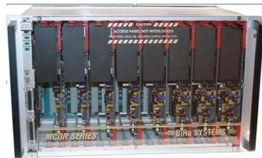
Figure 2: The Bira MCOR30 power converter board and Bira MCOR Crate2512.
