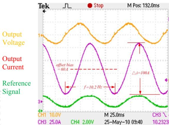
Figure 8: The program input sinusoidal waveform.
