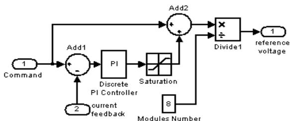
Figure 3: P-I compensator internal block diagram.
