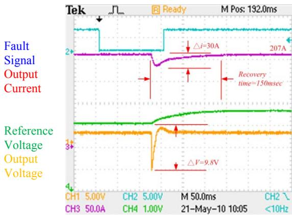
Figure 7: Relation between the fault testing signal and redundancy function.
