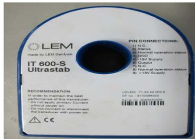
Figure 5: LEM IT 600-S Ultrastab DCCT.
