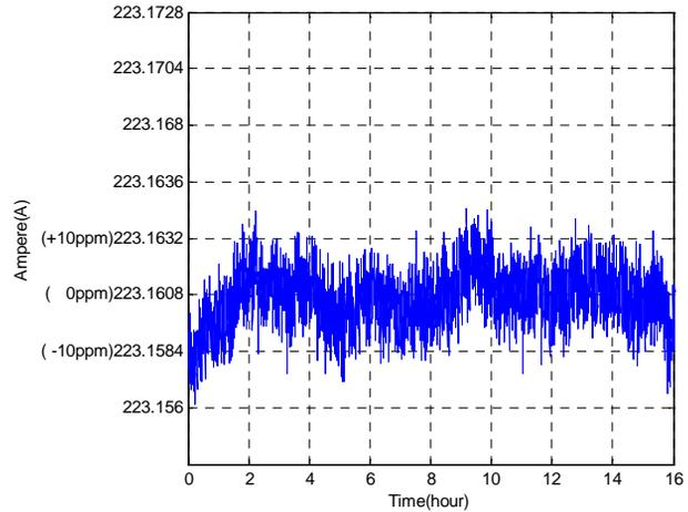
Figure 10: Stability of output current is setting 223.160A.
