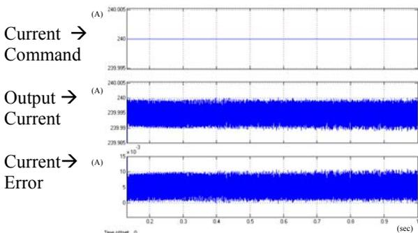
Figure 4: MATLAB simulink simulation result of P-I compensator.
