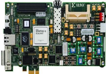
Figure 4:Xilinx Spartan-6 FPGA SP605 Evaluation Kit.
