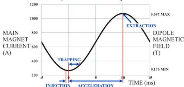
Figure 1: One cycle of the MMPS waveform.
