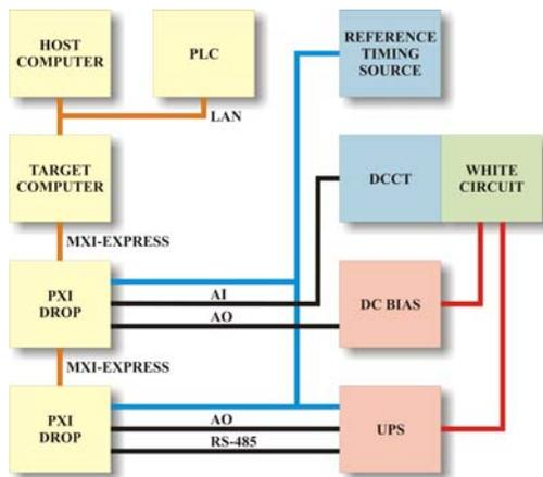
Figure 2: Control system hardware.
