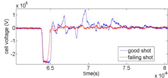
Figure 3: breakdown in oil
