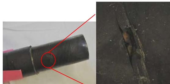
Figure 4: cable breakdown
