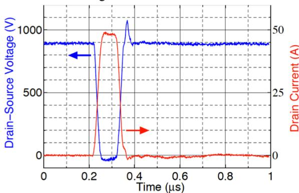
Figure 9: Voltage and current waveforms with a load resistance of 18.8 ohm.
