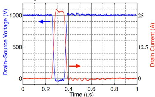
Figure 6: Voltage and current waveforms with charging voltage of 1 kV, repetition rate of 1 MHz, and load resistance of 37.5 ohm
