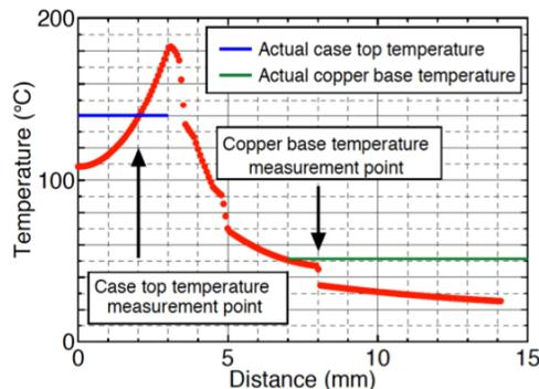
Figure 8: Temperature distribution along the centre axis of the device
