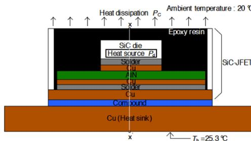
Figure 7: Thermal analysis model
