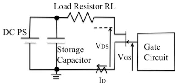
Figure 5: Experimental circuit
