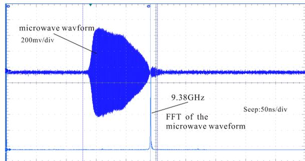
Figure 3: The microwave profile for the 9.38GHz high power microwave source
