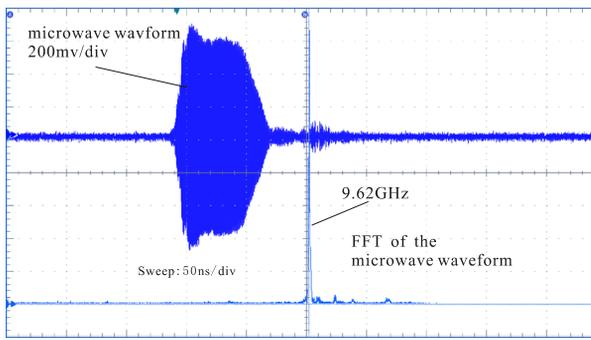
Figure 4: The microwave profile for the 9.38GHz high power microwave source
