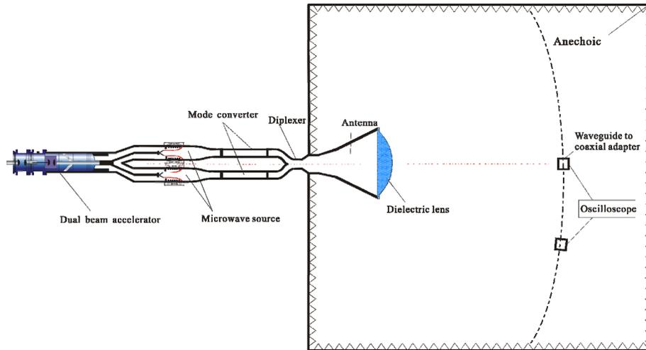
Figure 1: Schematic display of the microwave beating system.
