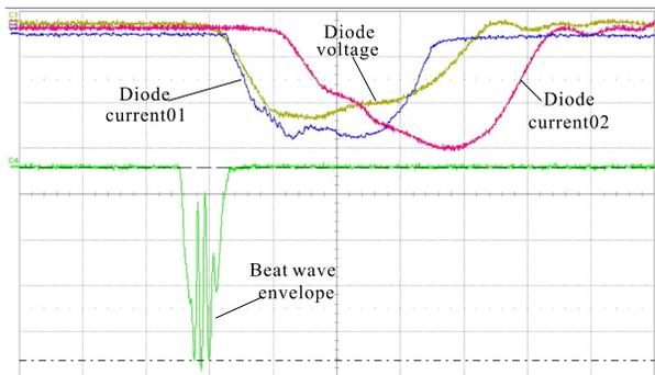
Figure 2: The diode current of the individual diode
