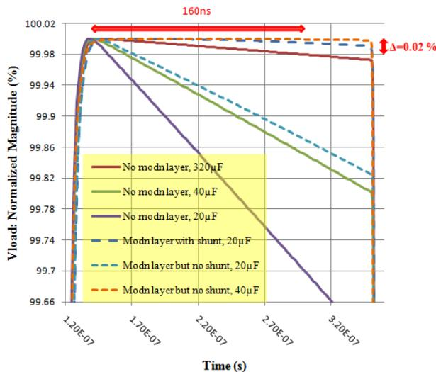
Figure 2: Simulation results for an inductive adder with different capacitances, with and without an analogue modulation layer.
