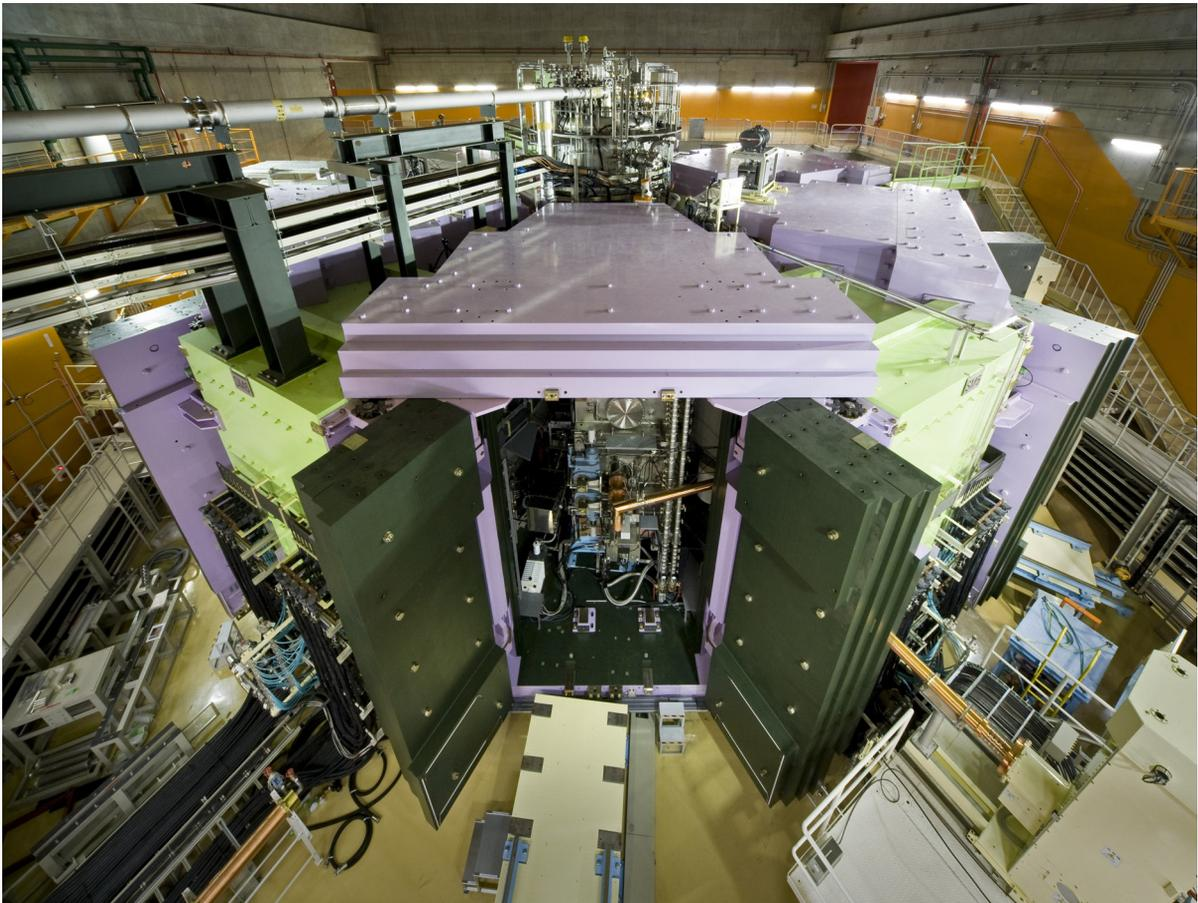
Photograph of the SRC when the side yoke shields are open. You can see the RF cavity inside.
